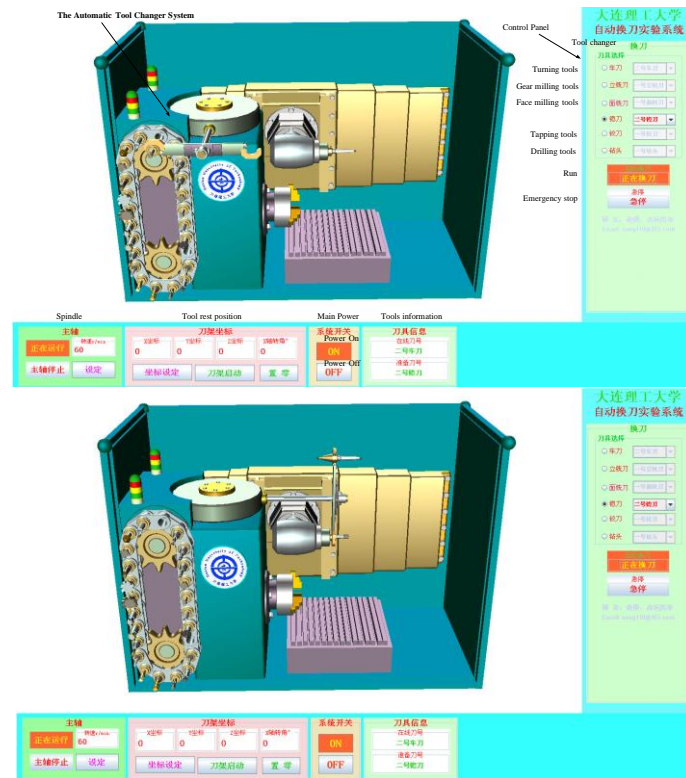
Figure 6. The Virtual Experiment Screenshot of Tool Changing Motion Control
