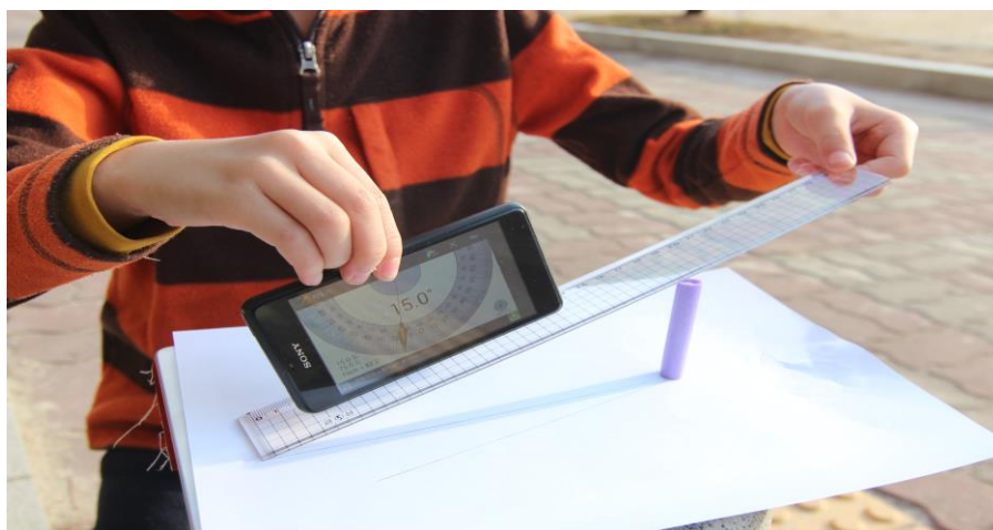
Figure 1. An Example of Method to Find Meridian Transit Altitude Using a Smartphone Application
